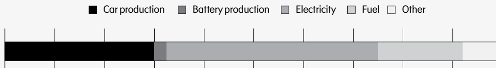
Emission split Lynk & Co 01 PHEV, combined mode with EU grid mix
